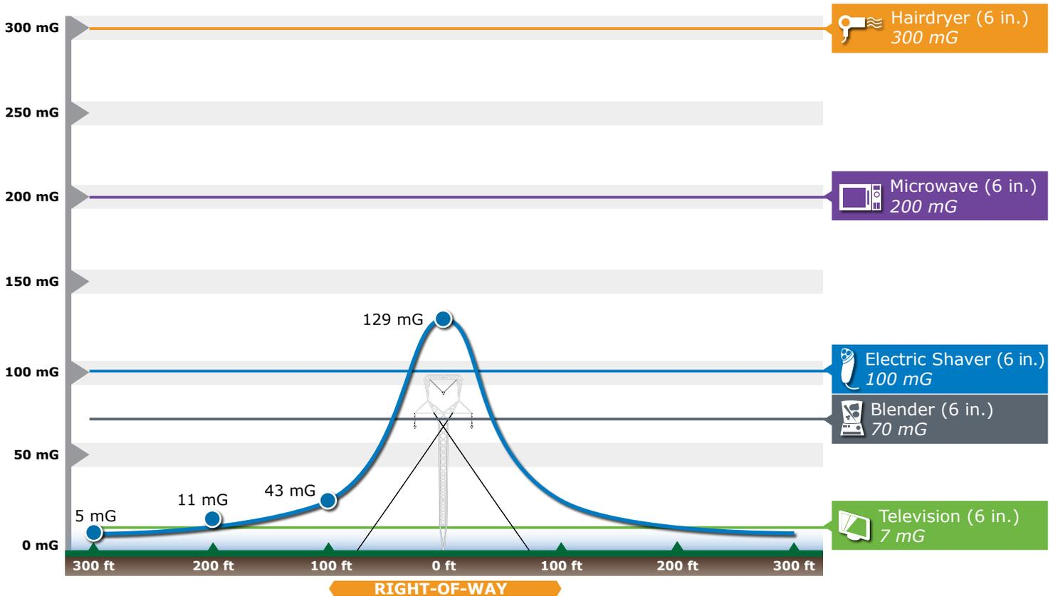
\*The figure above represents magnetic fields for a comparable 500 kV line and do not necessarily represent the measurements for the Great Northern Transmission Line.
